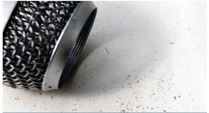
Gentle brushing with a toothbrush will remove dirt and other foreign matter adhered to the grille. Do this away from the body and sensitive microphone diaphragm.
